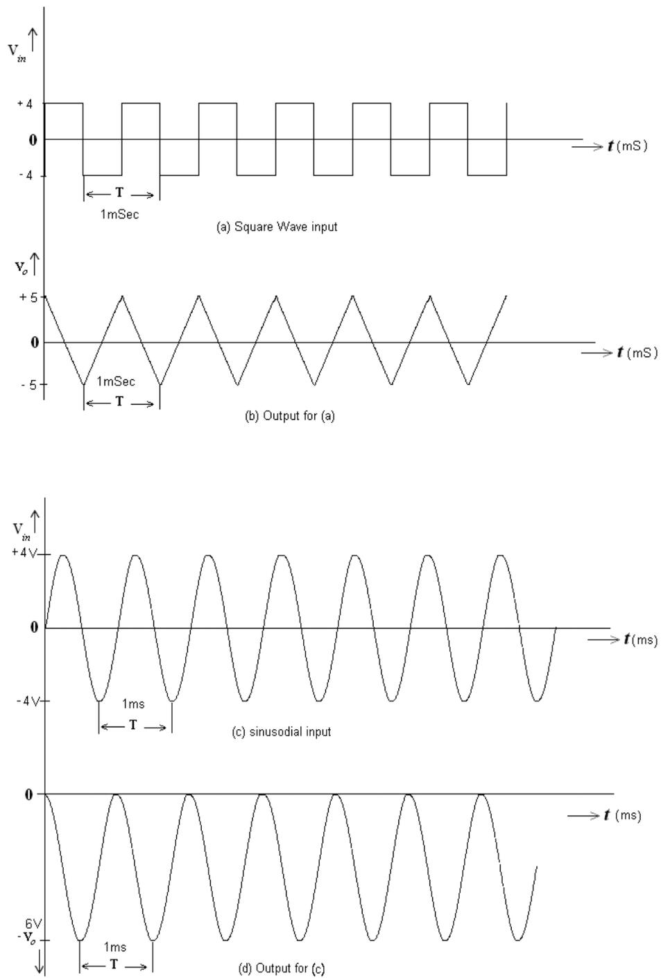
**Fig 4: Input and output waves forms of integrator**
