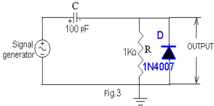
Negative peak clamping to  $V_r= -2v$
