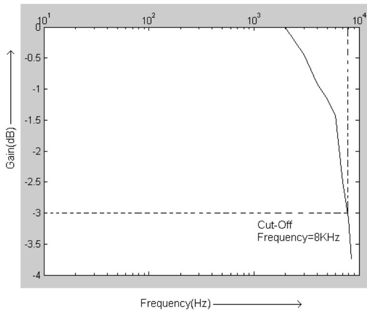
High Pass RC circuit frequency response:
