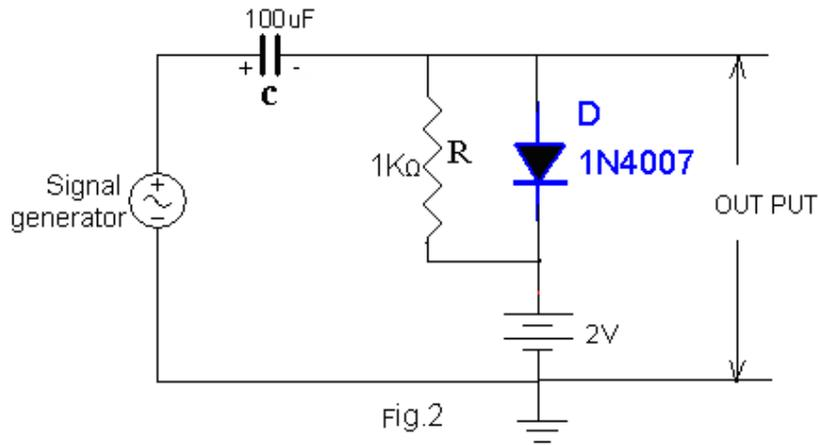
Negative peak clamping to  $V_r=0v$
