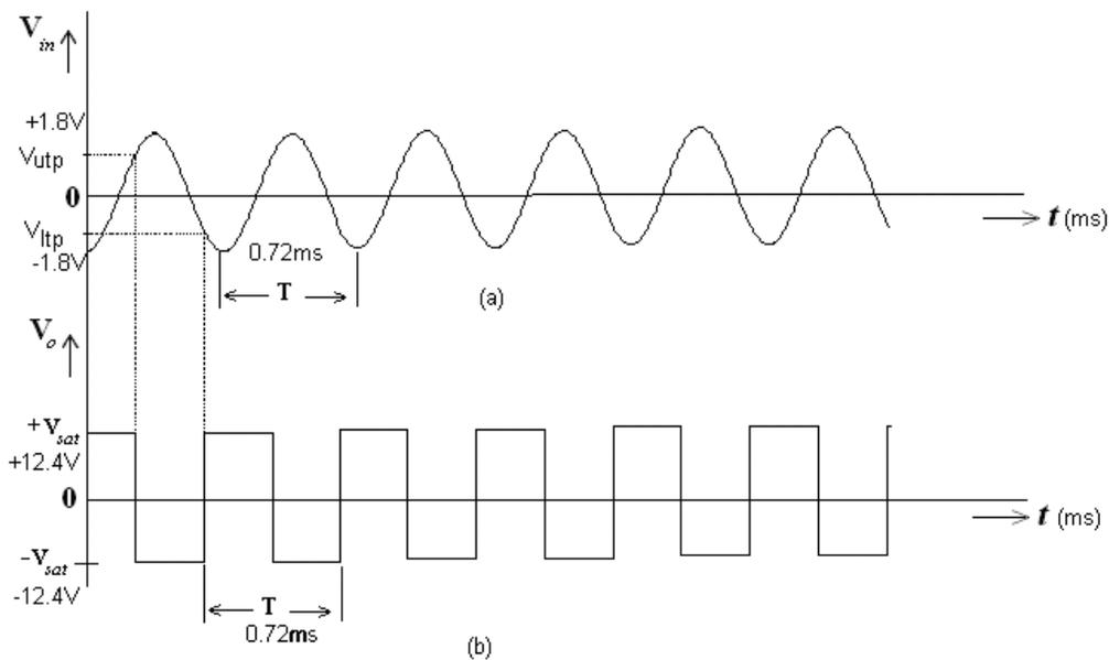
Schmitt trigger input wave form
