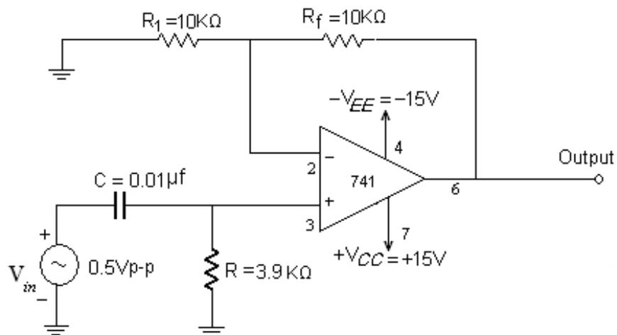
**Fig 2: High pass filter**
