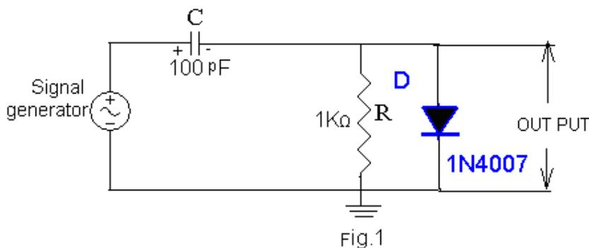
Positive peak clamping to  $V_f=2v$
