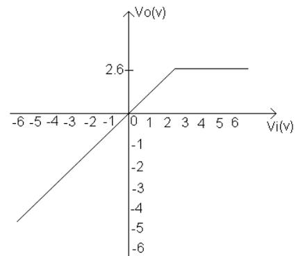
Positive base clipper: Reference voltage= 2V
