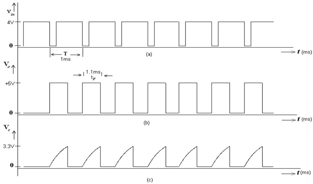
**Fig 3 (a): Trigger signal      (b): Output Voltage      (c): Capacitor Voltage**
