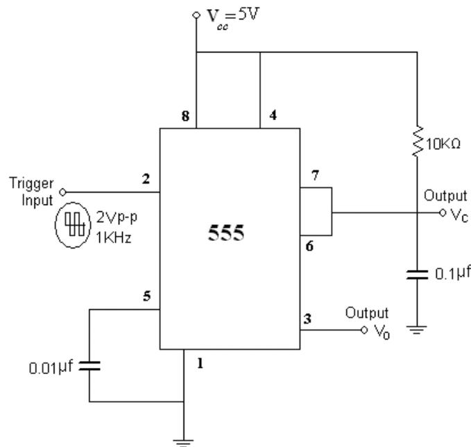
Fig 1: Monostable operation
