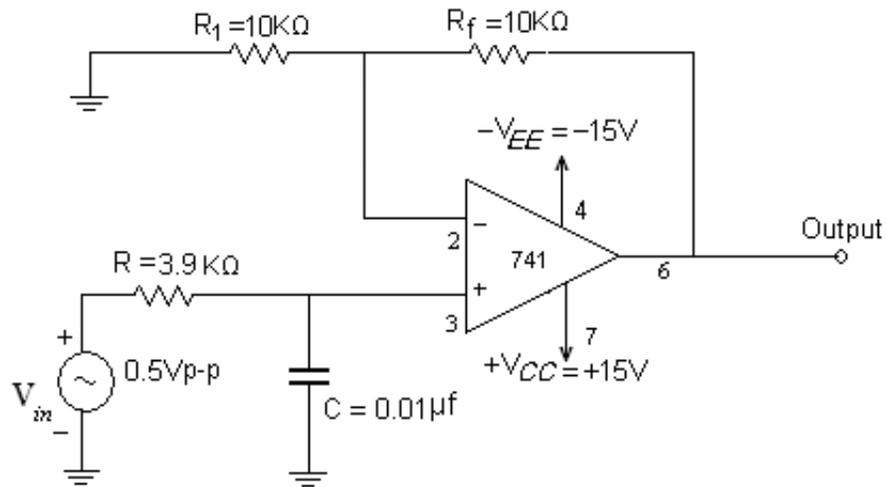
**Fig 1: Low pass filter**
