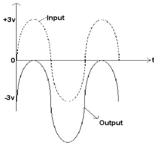
Positive peak clamping to  $V_r=2V$
