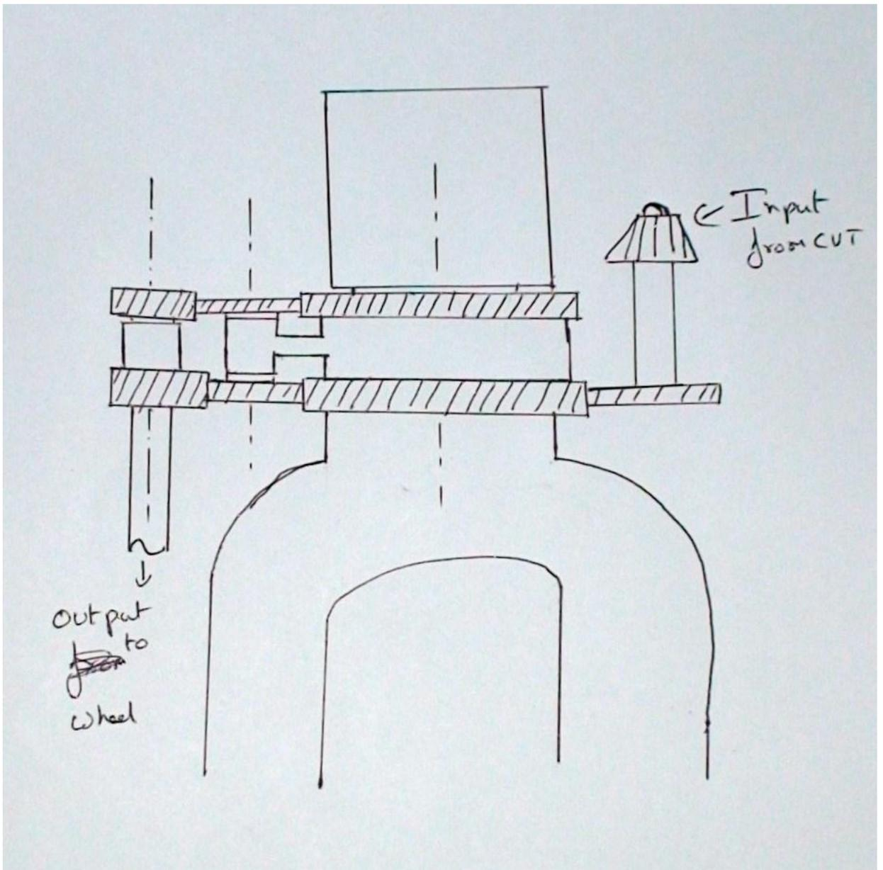
Figure 2 (transfer gear mechanism-front steering)
