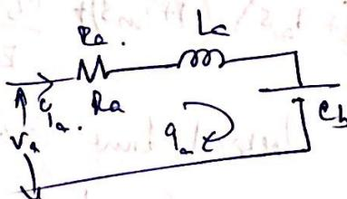
$$V_a - I_a R_a + l_a \frac{dI_a}{dt} + E_b = V_a \quad \text{--- (1)}$$
