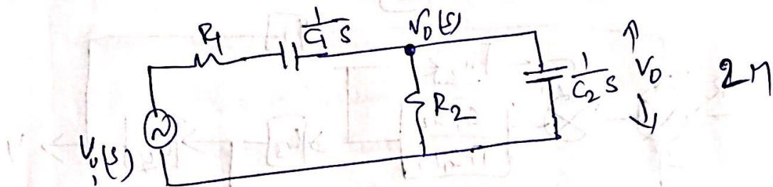
$$\frac{V_o(s) - V_i(s)}{R_1 + \frac{1}{C_1 s}} + \frac{V_o}{R_2} + \frac{V_o}{C_2 s} = 0 \quad \text{--- (1) } 1M$$
