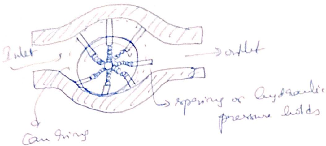
The rotor is offset with respect to the housing and the vanes constrained by can rings as they cross inlet and outlet ports.
