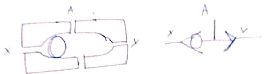
If pressure is applied to port  $X$  the ball is blown to the right blocking  $Y$  and linking port  $X$  and  $A$ . Similarly from other direction also.
