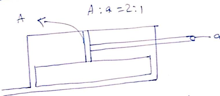
The cylinder with equal extension and retractive force
