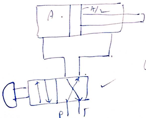
Cylinder with equal extension and retractive force
