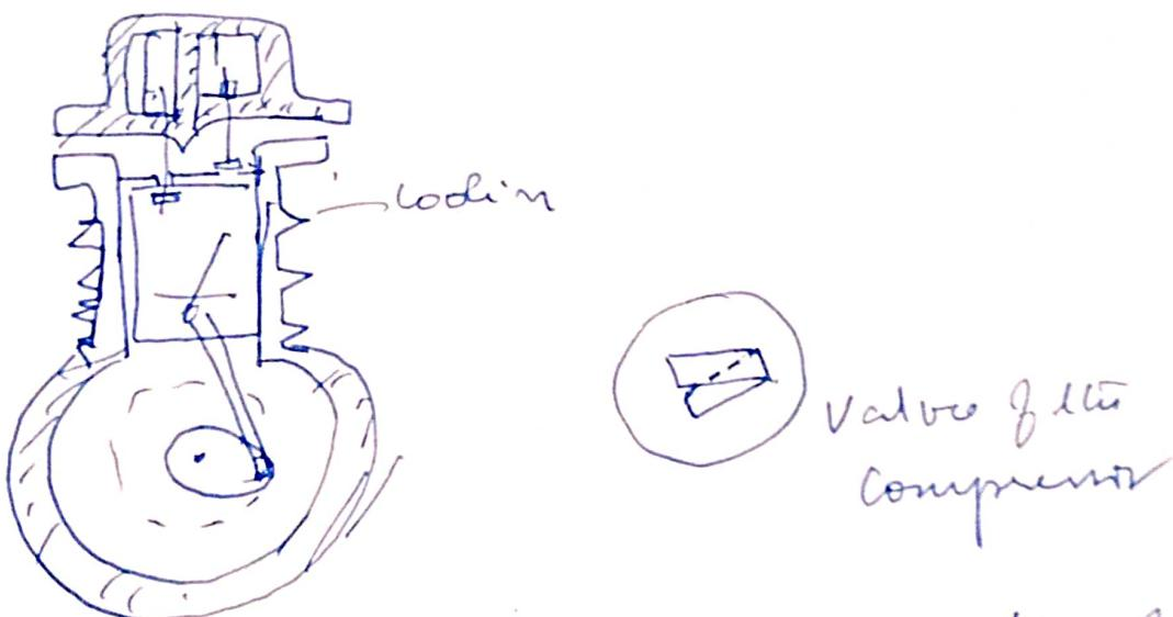
A compressor which produces one pulse of air per piston stroke is called single acting cylinder. On the other hand if it produces two pulses of air per piston strokes is known as double acting cylinder.
