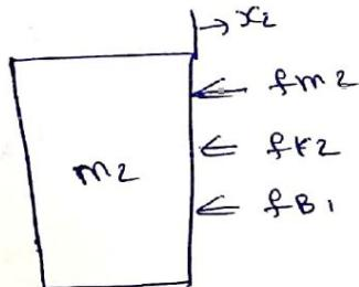
$$f_{m2} = m_2 \frac{d^2x_2}{dt^2}, \quad f_{k2} = k_2 (x_2 - x_1), \quad f_{B1} = B_1 \frac{d}{dt} (x_2 - x_1)$$
