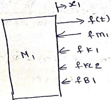
$$f_{m1} = m_1 \frac{d^2x_1}{dt^2}, \quad f_{k1} = k_1 x_1, \quad f_{k2} = k_2 (x_1 - x_2)$$
