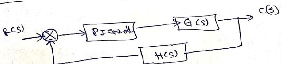
The PI-controller is a device that produces an output signal consists of two terms - one proportional to input signal and the other proportional to the integral of IIP signal.
