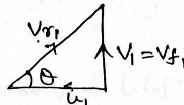
$$V_{f_1} = 10.47 \times \tan 20^\circ = 3.81 \text{ m/sec}$$
