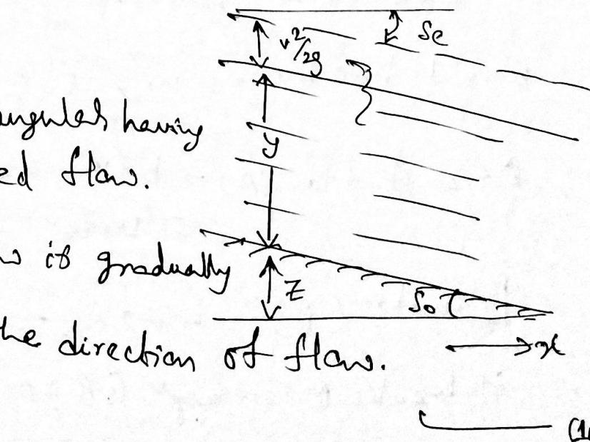
The energy equation at any section is given by B.E
