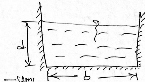
$$\text{Perimeter (P)} = b + 2d = 0.5 + 2(0.2) = 0.9 \text{ m} \quad \text{--- (1m)}$$
