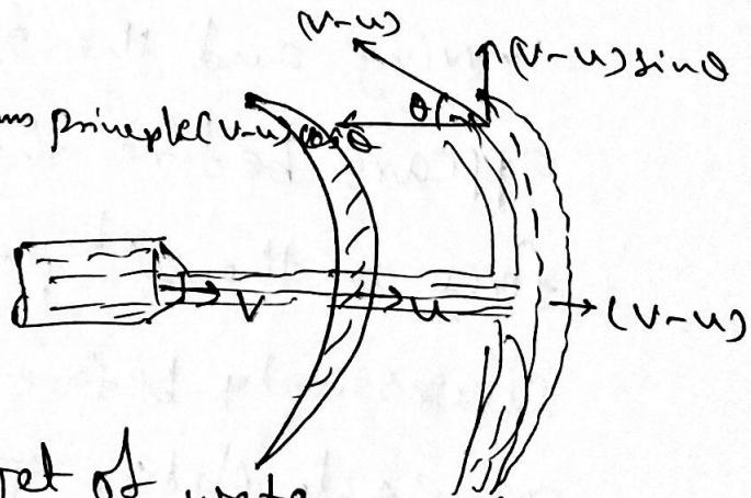
$\therefore$  force exerted by the jet of water on the curved plate in the direction of the jet ( $F_x$ )
