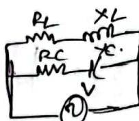
$$Y = \frac{1}{Z_L} + \frac{1}{Z_C}, \quad Z_L = R_L + j\omega L \quad Z_C = R_C - \frac{j}{\omega C}$$
