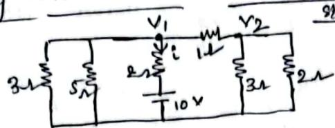
$$\text{by app Nodal analysis: } -\frac{V_1}{5} + \frac{V_1 - 10}{2} + \frac{V_1 - V_2}{1} = 0;$$
