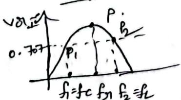
Bandwidth of system is range of freq for which current  $\pi_0$  volt is equal to  $70.7\%$  of its value at res. frequency.
