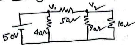
$$V_1 = 50; \frac{V_2 - V_1}{5\Omega} + \frac{V_2}{2\Omega} + \frac{V_2}{10\Omega} = 0;$$
