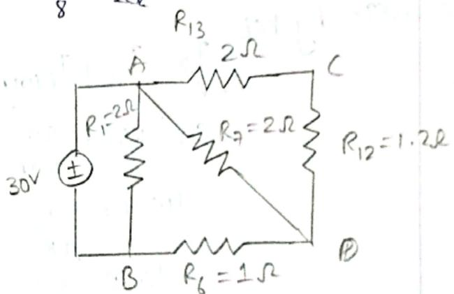
$$\textcircled{6} \quad 3.2\Omega \parallel R_7 = \frac{3.2 \times 2}{2+3.2} = 1.23\Omega$$
