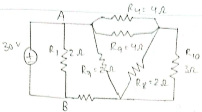
$$\textcircled{3} \quad R_8 \text{ & } R_{10} \text{ (Parallel)} = \frac{2 \times 3}{2+3} = \frac{6}{5} = 1.2\Omega$$
