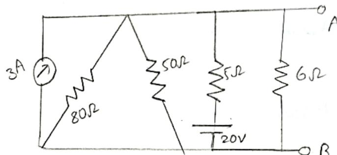
Sol: Convert a series combination of 20V, 5V into an equivalent circuit.
