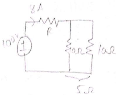
43) Determine the current in all three resistors in the circuit.
