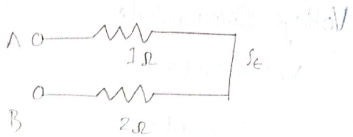
Because of short circuit the parallel resistance is to be neglected.
