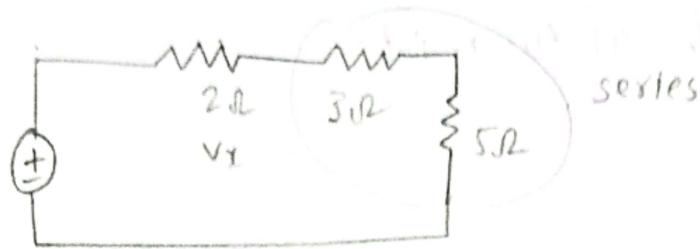
$$V_x = V_{2\Omega} = 10 \times \frac{2}{10}$$
