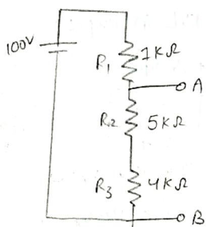
12.) Determine the current through each resistor in the circuit.
