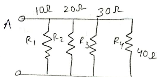
37.) Determine the current through Resistor  $R_3$ .
