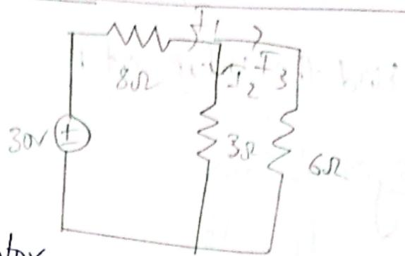
Step 2:- 8Ω is series with 2Ω resistor
