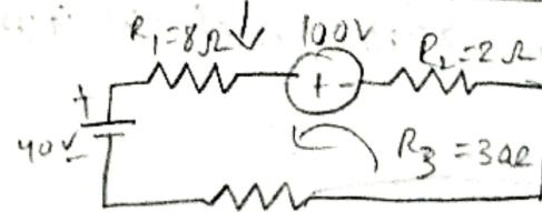
i) Determine the total amount of power in the circuit. Find the power absorbed by each resistor.
