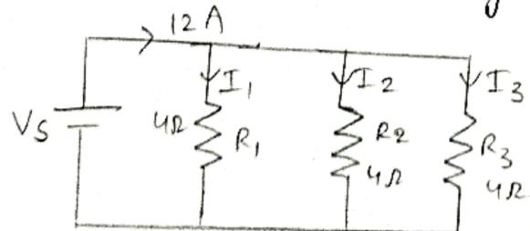
$$\text{Sol: } I_1 = I \cdot \frac{R_1 R_2}{R_2 + R_1} = \frac{12 \times 4 \times 4}{4+4} = \frac{24}{6} = 4A$$
