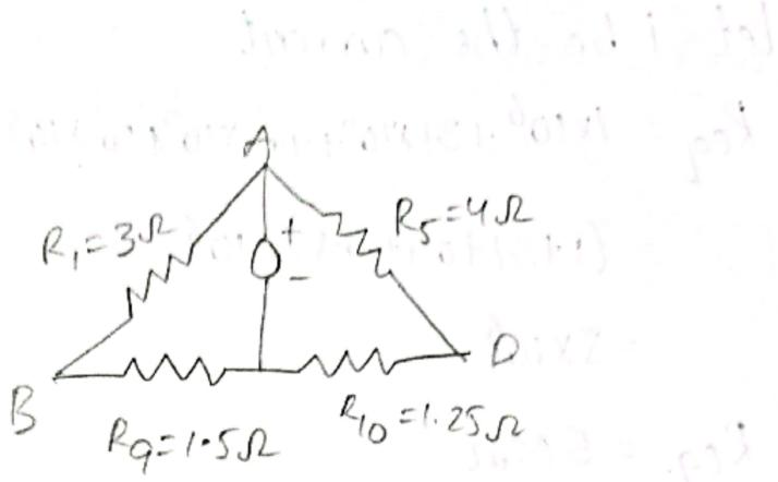
$$R_{11} \Rightarrow R_9 || R_1 = 1.5 + 3 = 4.5\Omega$$
