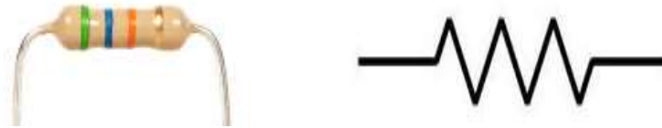
Fig 1: Resistor and its symbol.
