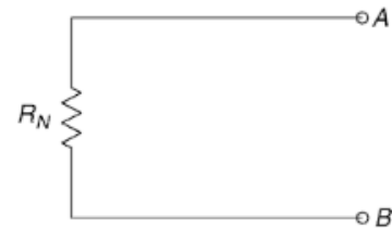
Fig. 3.256 Norton's equivalent network
