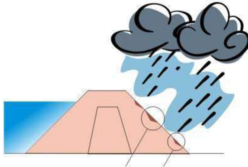
Figure 24. Scour of downstream face by impact of rain and resulting sheet flow
